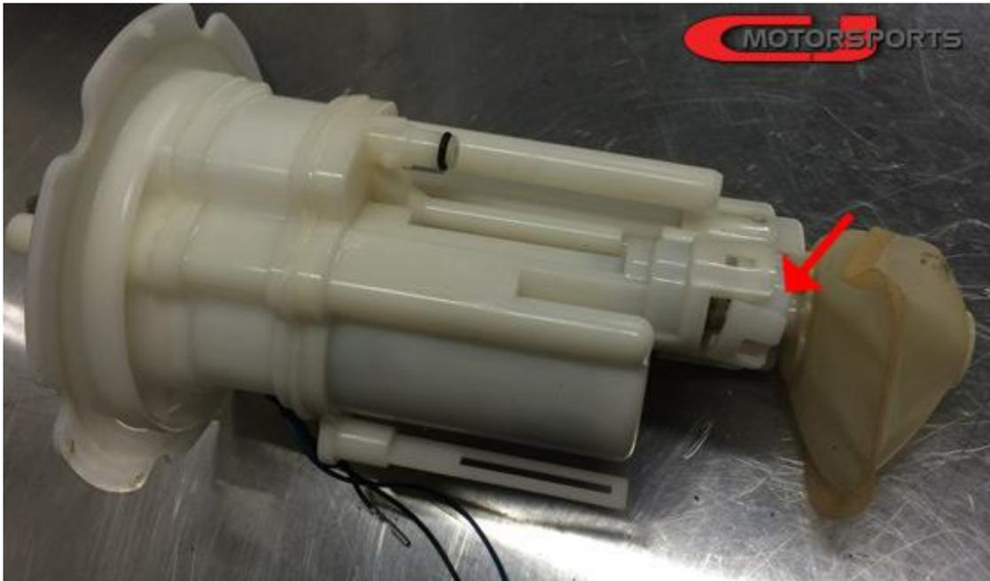
With the regulator exposed, pull it downward to remove.
