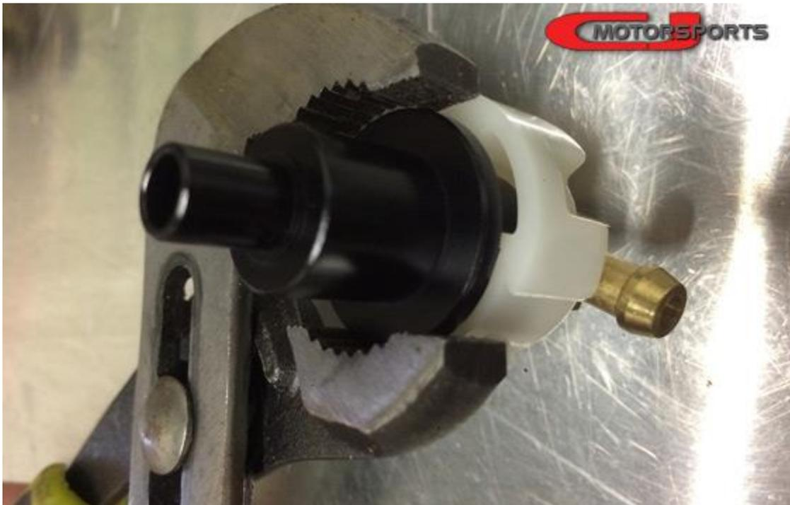
Install the supplied hose and clamp as shown. Slide the clamp halfway down the hose, push the hose onto the elbow fitting, and slide the clamp down to the end to tighten. It's a snug fit to get the clamp in there. Try and orientate the clamp as shown for vertical clearance.
