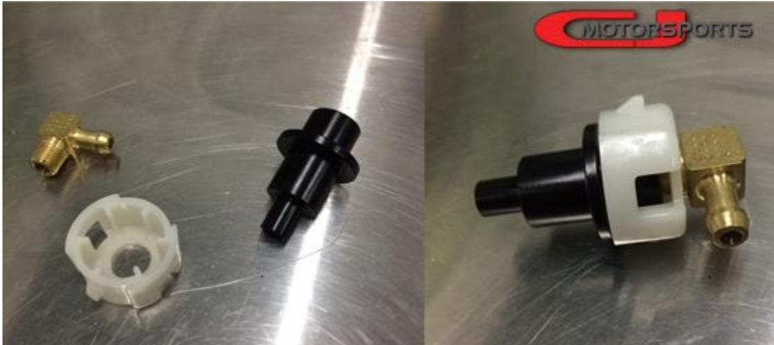
To tighten, you can hold the delete fitting by its largest diameter. This is not a sealing surface and any marring of the part will not affect its sealing. Tighten the elbow fitting with an adjustable wrench. This connection does not need to be extremely tight, just tight enough to get a decent seal. No thread sealant is necessary.
