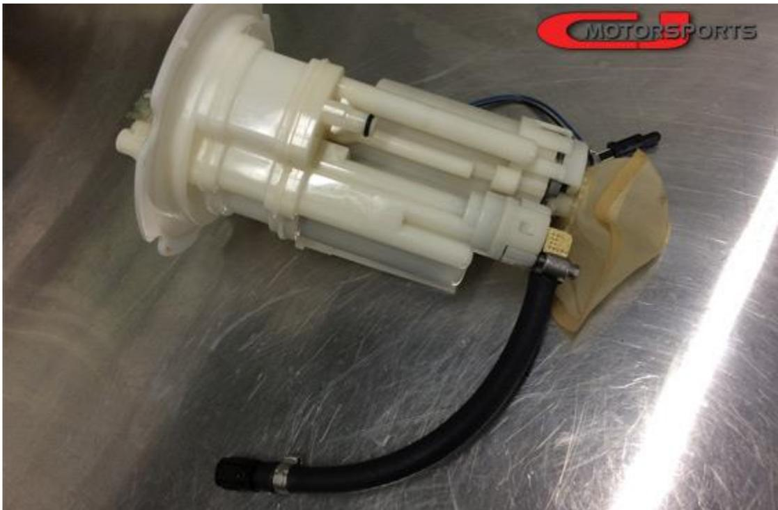
Using a rotary tool, grind away the structural webbing behind the electrical connector on the bottom side of the tank flange. Take care to make this area relatively smooth and flat to help ensure good sealing later.
