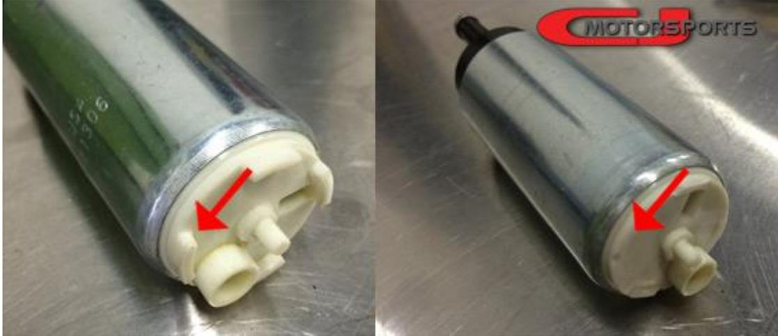
Carefully remove the fuel pump pickup from the factory fuel pump by using small pick tools to extract the metal retainer ring. Replace the fuel pump pickup to the new pump or install a new pickup. Install the metal retainer. Test fit the fuel pump into the housing by inserting the output barb into the receptacle of the pump housing and aligning the electrical connector.
