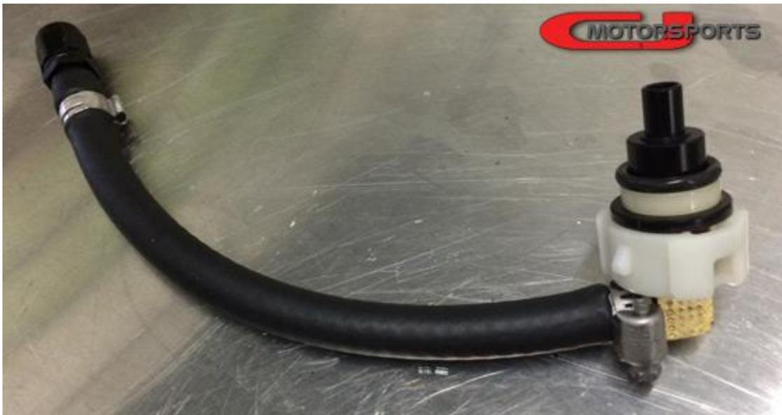
Install the CJM supplied o-ring into the regulator cavity.
