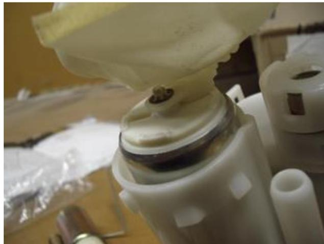
Check the fitment of the fuel pump retainer cap. With some pumps, you might find that it still needs modification to secure the taller pump. File down the example areas evenly until you are able to snap the fuel pump retainer back in place. When complete, plug in the electrical connector.
