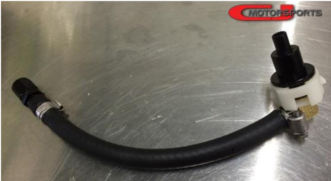
Install the plastic spacer and o-ring from the factory regulator onto the delete fitting.
