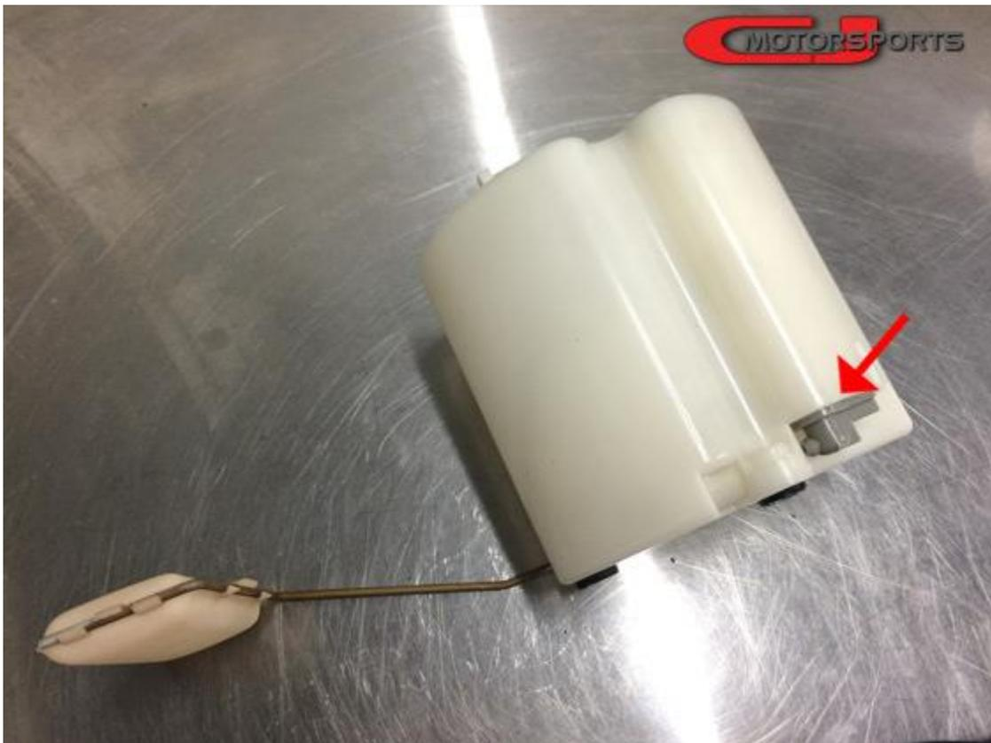
With the jet-pump removed, use a small drill to enlarge the pinhole outlet.
