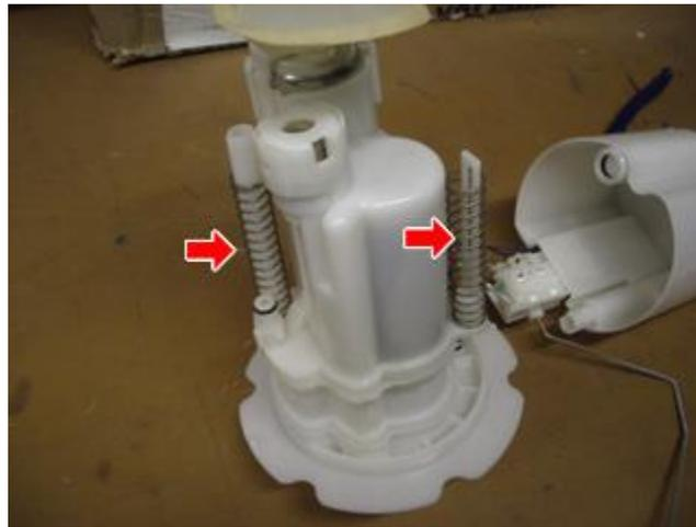
Compress the assembly until it snaps into the place. You may find that you need to lightly pull outward on this area of the canister to allow it to compress into position without interference.
