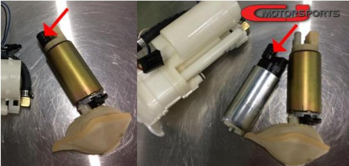
Many high output fuel pumps will be taller than the factory pump. In this case, you will want to make the pump as short as possible to assist reinstalling the retaining cap.
