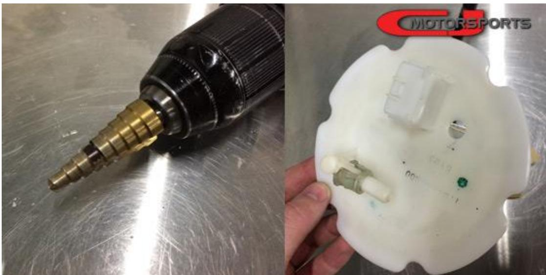
Install one of the seal washers to the bulkhead fitting, and insert the fitting into the tank flange.
