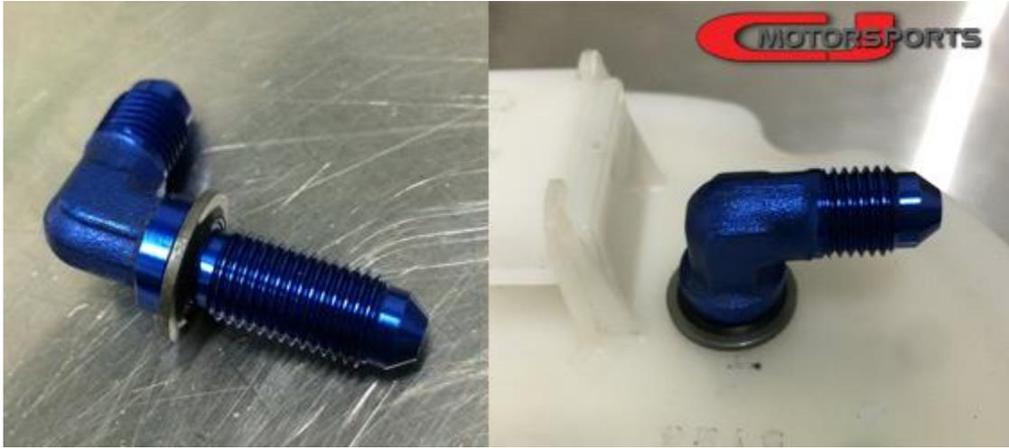
Install the second seal washer to the bulkhead fitting on the inside of the tank flange, and thread on the bulkhead nut.
