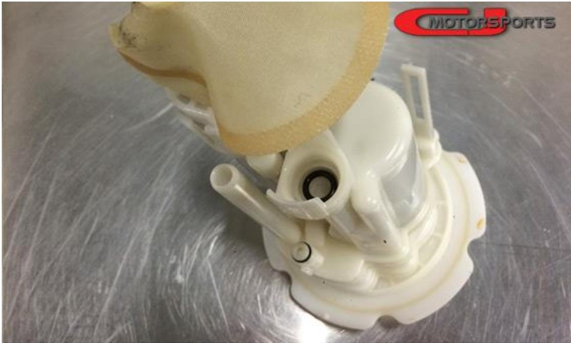
Install the delete fitting assembly into the cavity, making sure both o-rings stay in place. Check that the cap is secured in place by both locking tabs.
