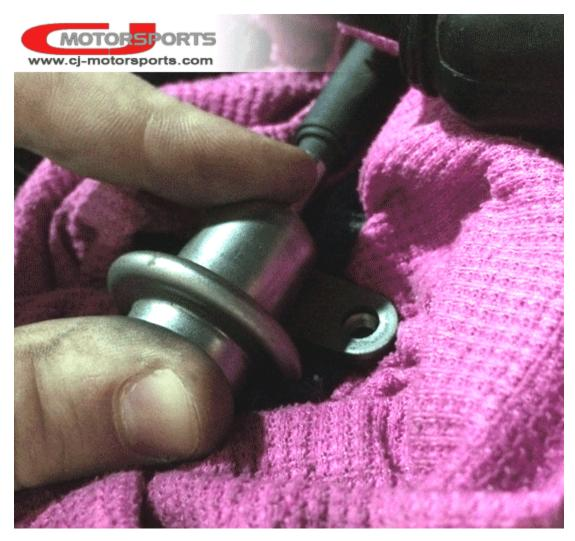
Continuously apply downward pressure to prevent the damper from lift-off while covering the rest of the area with rags.
