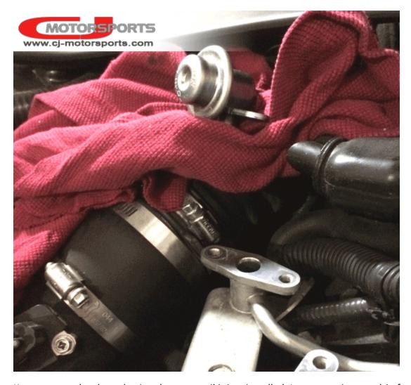
Keep a rag under the pulsation damper until it is reinstalled. It may continue to drip for a while.
