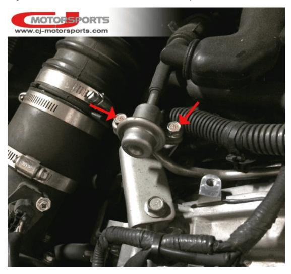
Stuff shop rags around and underneath the 2 bolt flange of the pulsation damper. Tuck them in well to absorb all the fuel that will discharge when the damper is lifted.
