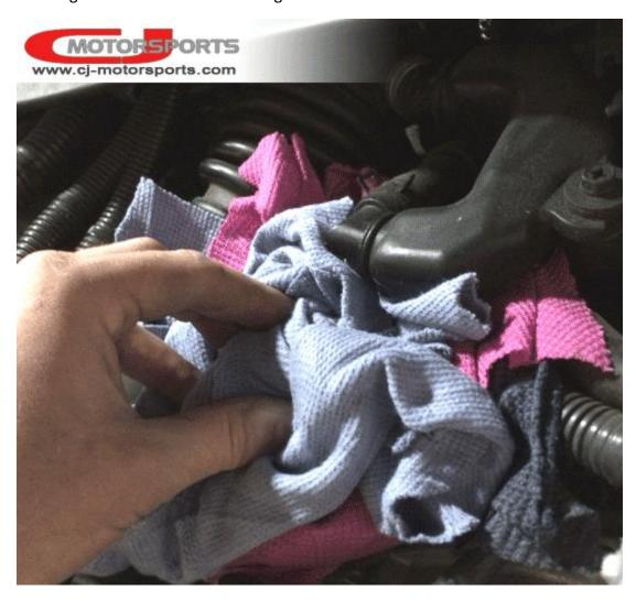
When satisfied with rag coverage, you may slowly relieve pressure from the damper and begin to apply upward pressure on it. It will need to raise about ¼" up before the o-ring will begin to exit the bore and allow fuel to escape. You will hear it, and you will feel it soaking into the rags. It is recommended to relieve pressure in a controlled manner rather than all at once. You can let out a little at a time several times until there is no longer any pressure.
