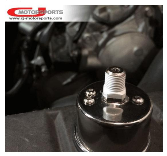
Thread the gauge into the billet spacer block until hand tight. Use the 7/16 wrench on the square nut at the base of the gauge to further tighten until the gauge is upright.
