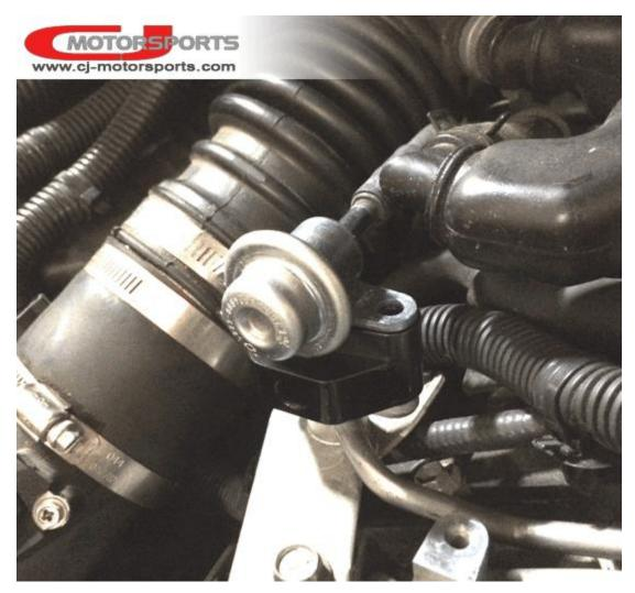
Install the supplied 5mm hex bolts with washers to secure the damper to the fuel inlet tube, sandwiching tight the billet spacer block.
